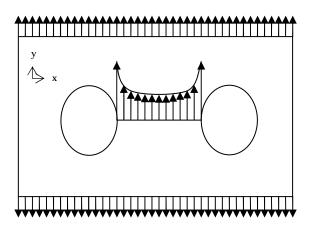
Figure 14.2: Stress concentrations around cut-outs loaded in tension
